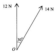
Two horizontal forces act at the point O. One force has magnitude 12 N and acts along a bearing of  $000^{\circ}$ . The other force has magnitude 14 N and acts along a bearing of  $030^{\circ}$  (see diagram).
