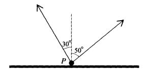
A particle P of weight 30 N rests on a horizontal plane. P is attached to two light strings making angles of  $30^{\circ}$  and  $50^{\circ}$  with the upward vertical, as shown in the diagram. The tension in each string is 15 N, and the particle is in limiting equilibrium. Find
