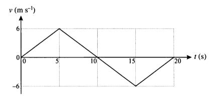
An athlete runs in a straight line from point A to point B, and back to point A. The diagram shows the (t, v) graph for the motion of the athlete. The graph consists of three straight line segments.
